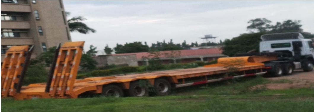
Picture 20: Procured Lowbed Truck (75 Tones) at National Steel Raw Material Exploration Agency, Kaduna
